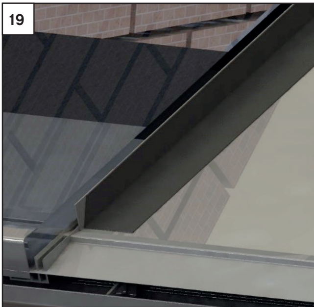
Lay membrane across rest of WARMroof, leaving extra at glass to lap up behind soaker rail. Take soaker rail with the ripped down upstand (approx. 25-30mm) and position tight up to edge of panels/ back of PVC thermal break. (Note: glazing bar end cap omitted from this view for clarity)
